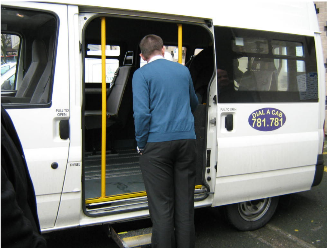
Shows “tail board” and marking to stop passengers standing on rear of vehicle
